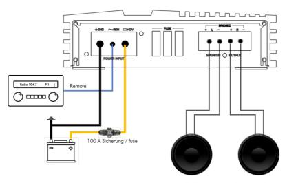
Geringste Lautsprecherimpedanz je 2  $\Omega$  Minimum speaker impedance 2  $\Omega$  each
