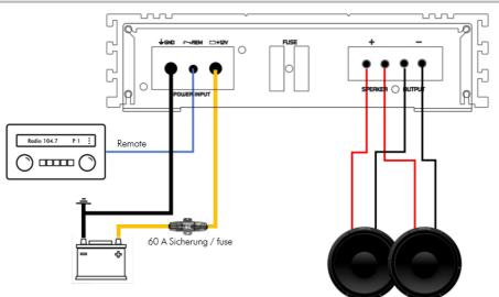
Geringste Lautsprecherimpedanz je 2  $\Omega$  Minimum speaker impedance 2  $\Omega$  each
